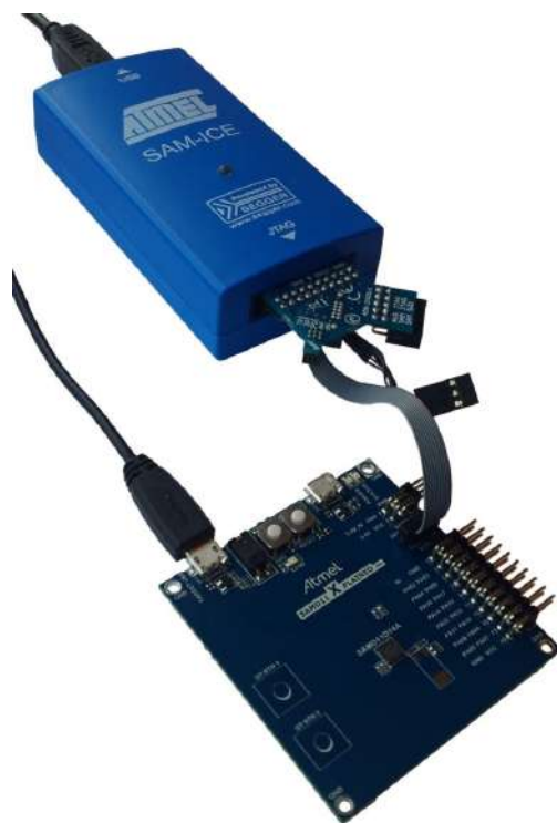
Figure 5-7. SAM-ICE using an Atmel-ICE Adapter
