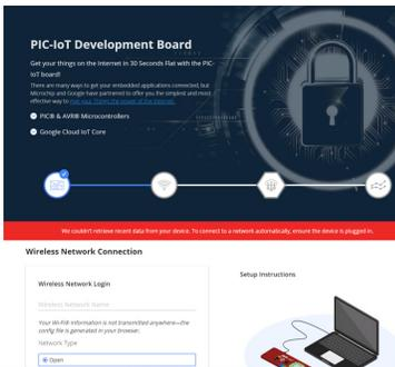
Drag and drop the downloaded **WIFI.CFG** file to the **CURIOSITY** drive. Your board will blink, and automatically connect to the network.
